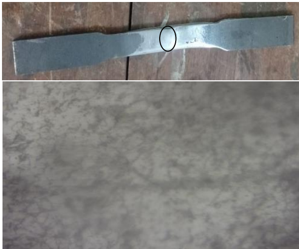
Gambar 1. Hasil uji mikro media air garam
